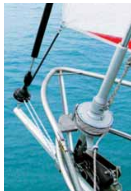
When the sail is unrolled RollGen does not interfere with any manoeuvres.
