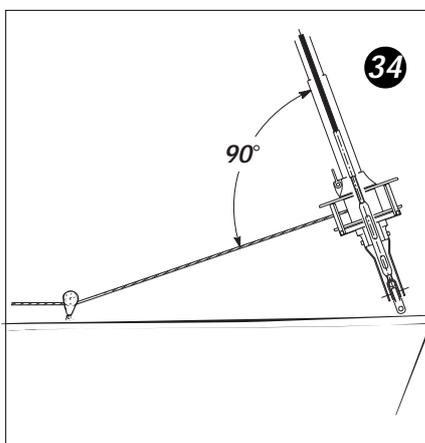
■ C-9 Attaching the furling line to the drum
